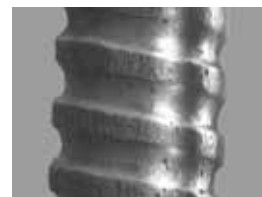
FIGURE 6 Excavated from mud dredged from a canal in Delft, this portion of the screw thread from the Camacho/Pallas microscope is unlike any of the recent attempts to produce replica microscopes. Imaged with the Hitachi S-3400N at 40x and an accelerating voltage of 8 kV, this macrograph helps us to characterise Leeuwenhoek's instrument.
