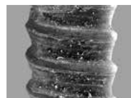
FIGURE 11 Distorted industrial dies have been used to create non-standard screw threads, as in this example from the Boerhaave museum. Here the profile is not comparable with an industrial standard, though the parallel scoring reveals this thread was cut with a die, and not rolled. In a case of this sort, only the SEM can provide conclusive evidence.
